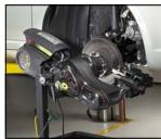
**ALWAYS** measure rotor before and after a brake job
